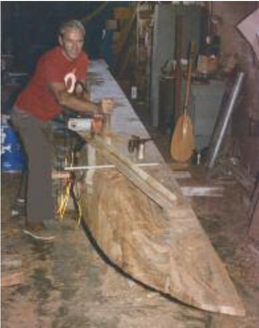
Joe Quigg uses a chain saw to shape a 200-year-old koa log into the canoe Kaoloa .
