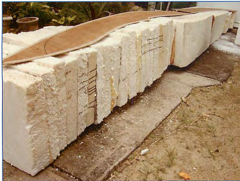
The ama started with chunks of old boogie boards and fish coolers.
